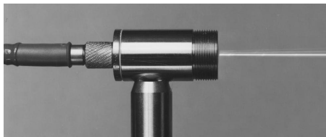
Fig. 4. Optical head of a low-power UV passively Q -switched microchip-laser system packaged in a 1-cm-diameter \times 2.5-cm-long stainless steel can.
